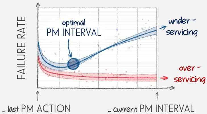
Most analyses we have completed show machines are chronically OVER-SERVICED, making the blue post-PM failure rate above very rare. This means that many machines can be SERVICED LESS and IMPROVE RELIABILITY. It should also be noted that there is ALWAYS MAINTENANCE-INDUCED failure, as shown by the initial (and temporary) increase in failure rate.
